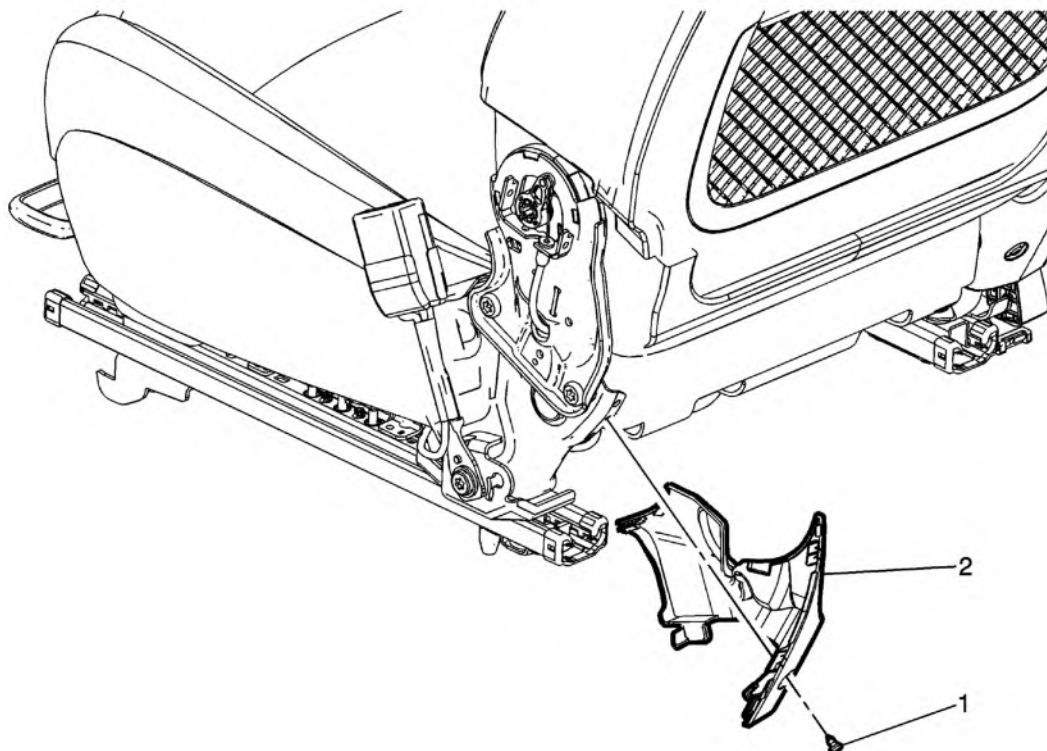
Fig. 20: Passenger Seat Inner Recliner Finish Cover (Inboard With AG5). Courtesy of GENERAL MOTORS COMPANY
